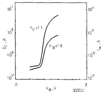
Fig. 4 Room-temperature Gummel plot of carbon-doped InGaP/GaAs/InGaP DHBT
