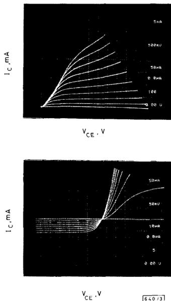
Fig. 3 Room-temperature common emitter characteristics of InGaP/GaAs/InGaP DHBT with  $14 \times 40 \mu\text{m}^2$  emitter area
