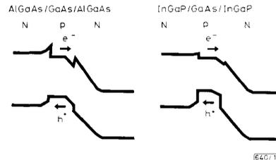
Fig. 1 Schematic diagrams of AlGaAs/GaAs/AlGaAs and InGaP/GaAs/InGaP double heterojunction bipolar transistors
