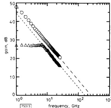
**Fig. 3** Current gain and Mason unilateral power gain against frequency for 0.08 μm-gate InAs-inserted-channel HEMT with gate width of 50 μm
