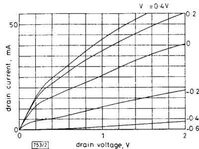
**Fig. 2** Current-voltage characteristics of 0.08 μm gate InAs-inserted channel HEMT with gate width of 50 μm
