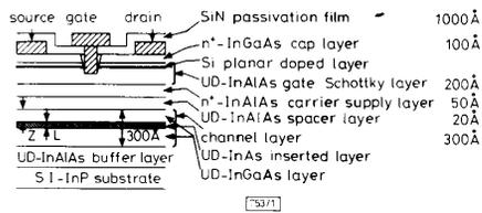
**Fig. 1** Device structure of InAs-inserted-channel HEMT
